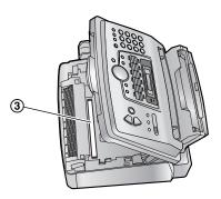
**9** Close the front cover (①) by pushing down on both sides, until locked.
